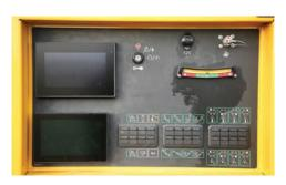
**COMPLETE CONTROL.** Optimize productivity and flexibility when operating with these two features: An industry leading, full function, wireless remote control lets you, from the cab, adjust machine settings as conditions change, including control of the infeed settings, vacuum settings, shaker table, conveyor height and more. The 7-in (18-cm) onboard color touch screen display shows machine data and allows you to intuitively set up the machine for maximum efficiency.
