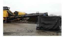
EFFECTIVELY CONTAINS TRASH. The CS3500 collects contaminants and puts them on one trash conveyor that's 36-in (91-cm) wide and can reach up to 16-ft (4.9-m) high. The trash conveyor allows the operator to discharge into dumpster containers, trucks or simply make a large pile.
