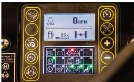
**KNOWLEDGE ON DISPLAY.** An integrated system display toggles through machine diagnostics, including engine rpm, fuel level, alternator voltage, engine coolant temperature and engine hours. When in either ground drive or using a rear attachment, the display indicates the percentage of the hydrostatic capacity being utilized, allowing the operator to easily monitor important machine functions.
