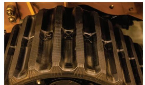
**QUAD TRACK SYSTEM.** The quad track system offers improved flotation, reduced surface damage and increased tractive effort. Four-wheel steer and crab steering are functional with both quad track and rubber tire options.
