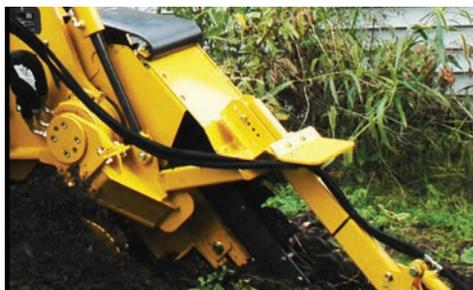
**MAKE SENSE OF YOUR TRENCH.** When difficult conditions are encountered while trenching, causing a sudden drop in engine speed, the TrenchSense™ electronic control system automatically pauses the forward motion of the tractor to prevent engine shutdown and recalibration of the machine controls. Once preset engine and trencher speed recovers, forward auto creep resumes. The sequence occurs within seconds and requires no operator adjustment.
